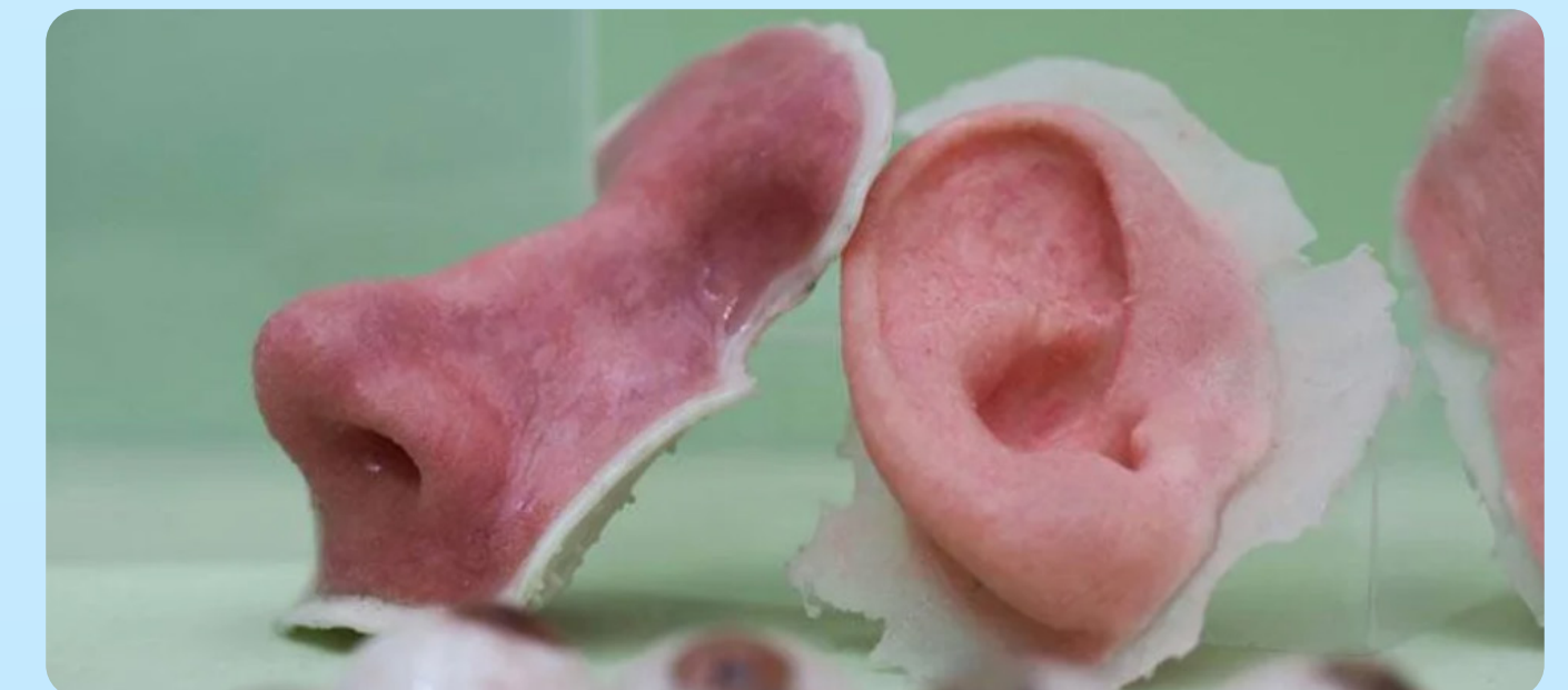
Nose and ear 3D printed from live tissue. Source: The future of Things
